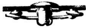
QUARTER TURN SPIRAL CAM FASTENER STUD WITH SPIRAL CAM AND MATING SPRING (COURTESY DZUS FASTENER COMPANY, INC.)
