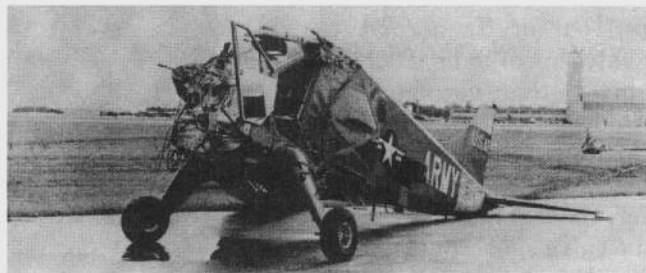
Figure 31-7. Failure to Color Code Aileron Control Chains Caused This Accident
