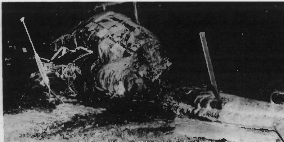
Figure 37-24. Design Vent Lines To Traverse All Directions of a Fuel Tank To Minimize Post-Crash Fires (Ref. 1)
