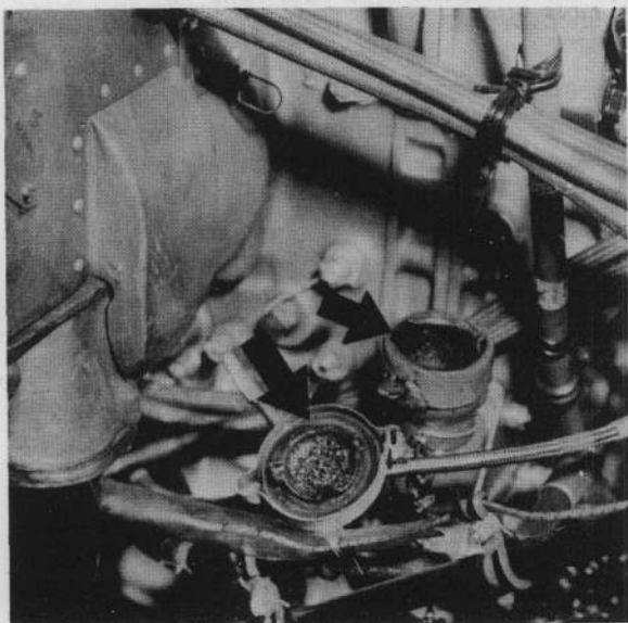
Figure 31-25. Design Oil Filler Cap To Prevent Loss in Flight (Ref. 1)
