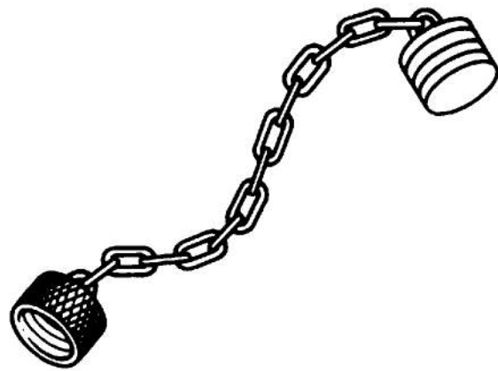
Figure 21-25. Use of Chain Prevents Loss of Small Removable Parts
