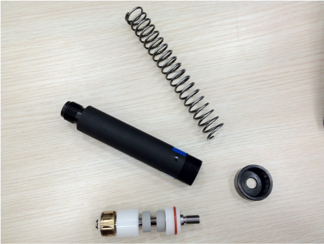
Figure 5-2: Disassembled Off-The-Shelf Shock Absorber
