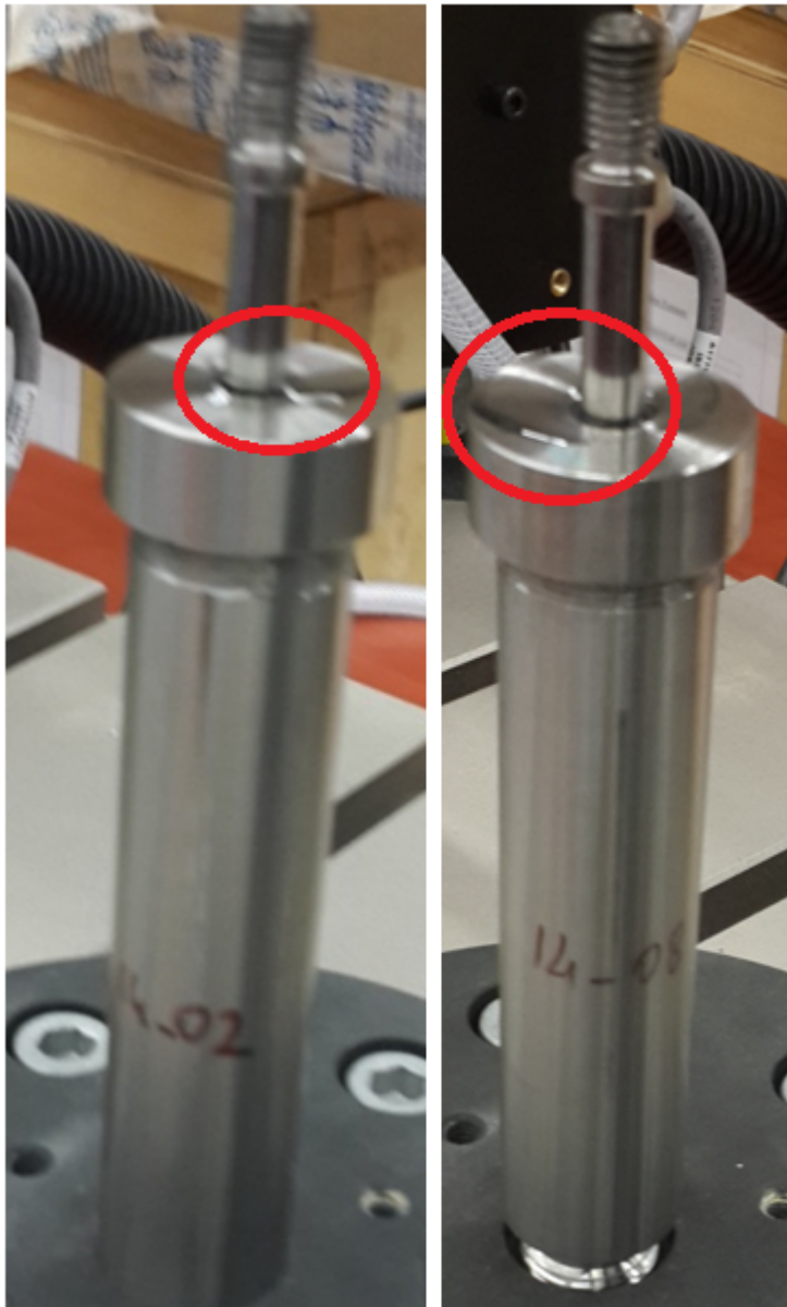
Figure 5-5: Leakage of Viscous Oil from Pistons P1402 and P1408
