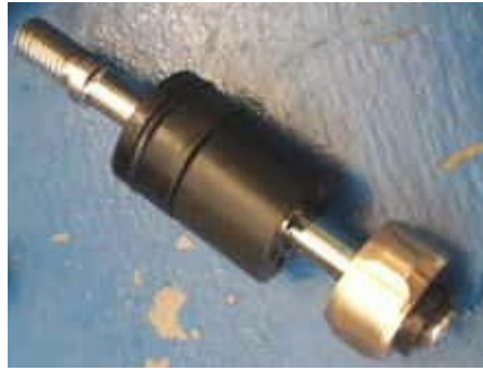
Figure 5-6: Seal Cap Assembly Manufactured from Teflon®
