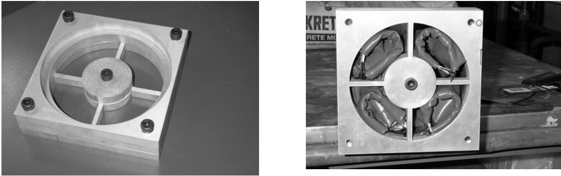
Figure 5.4 Cast fixture (a) and closed of “damping sausages” (b)
