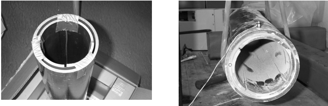
Figure 5.2 Split tube, before (a) and after (b) epoxy filling
