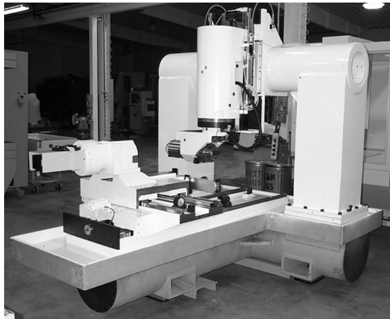
Figure 6.1 STG 5-axis tool and cutter grinder
