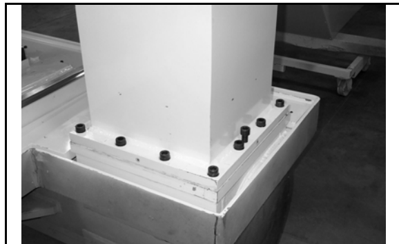
Figure 3.6 STG bridge - base joint
