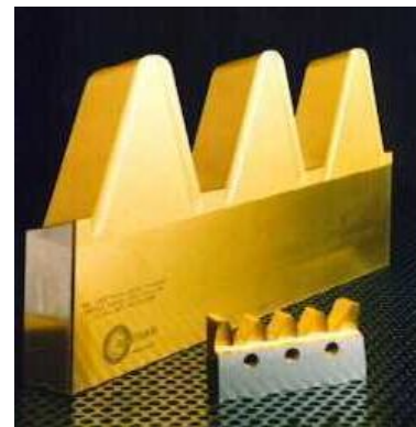
Fig. 19.4. Standard rack dimensions and the basic rack tool form [Doug Wright UWA]
