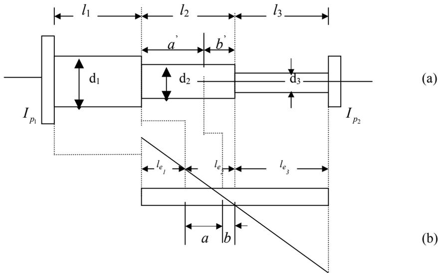
Figure 2.7(a) Two discs with stepped shaft (b) Equivalent uniform shaft
