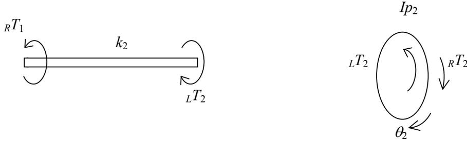
Fig. 2.9(a) Free body diagram of shaft section 2
