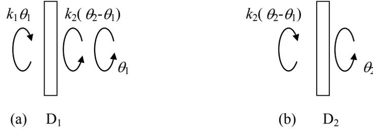
Figure 2.12 Free body diagram of discs
