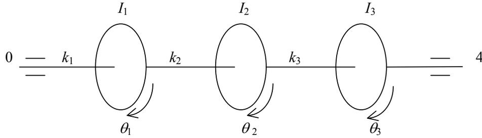
Figure 2.8 A multi-disc rotor system
