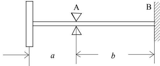
Figure E2.1 An overhang rotor system
