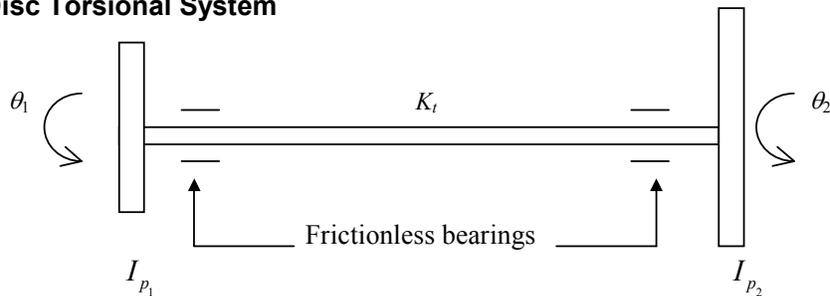
Figure 2.3 A two-disc torsional system
