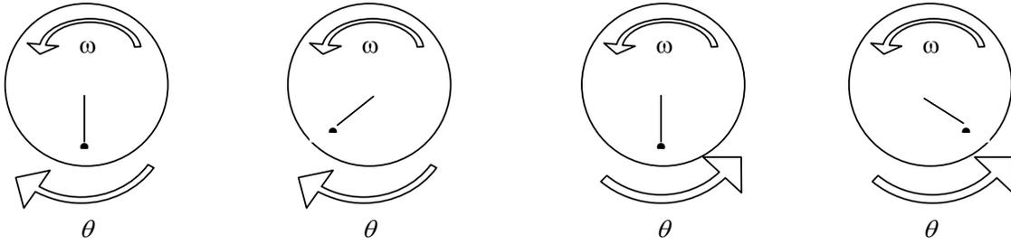
Figure 2.2 Torsional vibrations of a rotor
