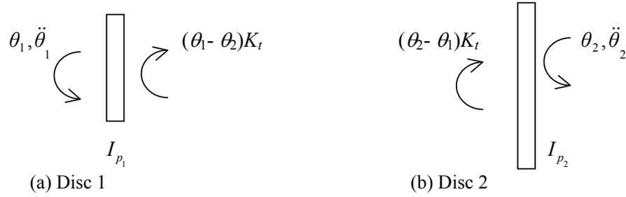
Figure 2.4 Free body diagram of discs
