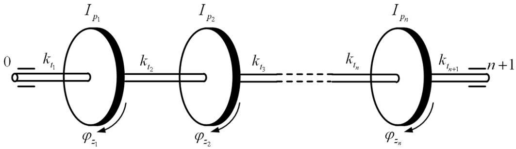
Figure 6.18 A multi-disc rotor system
