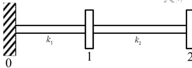
Figure 6.29 Two-discs rotor system with numbering of stations
