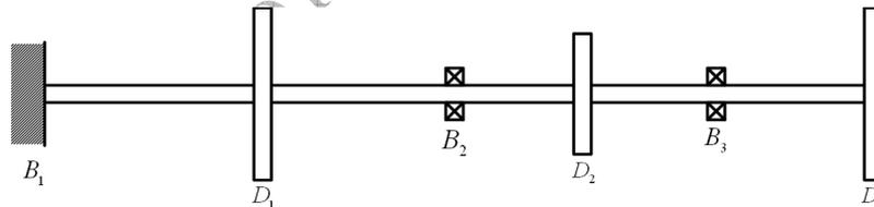
Figure E6.4 A multi-support multi-disc rotor system
