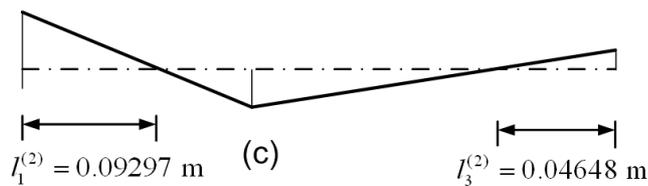
Fig. 6.17 (a) A three-mass rotor system (b) single node mode shape (c) two node mode shape
