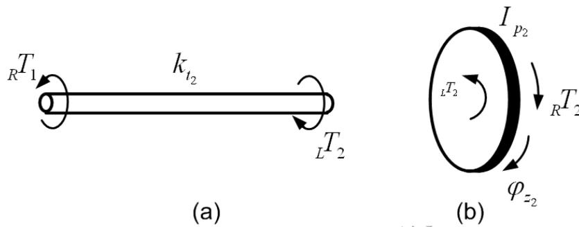
Fig. 6.19(a) A free body diagram of shaft section 2 (b) A free body diagram of rotor section 2
