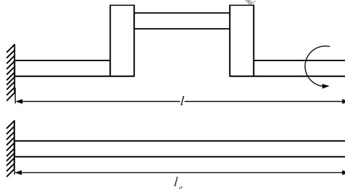
Figure 6.52 Equivalent length of a crank
