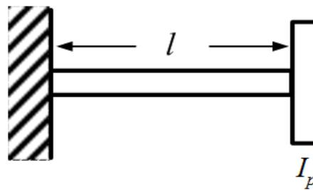
Fig 6.25 A shaft with cantilevered end conditions
