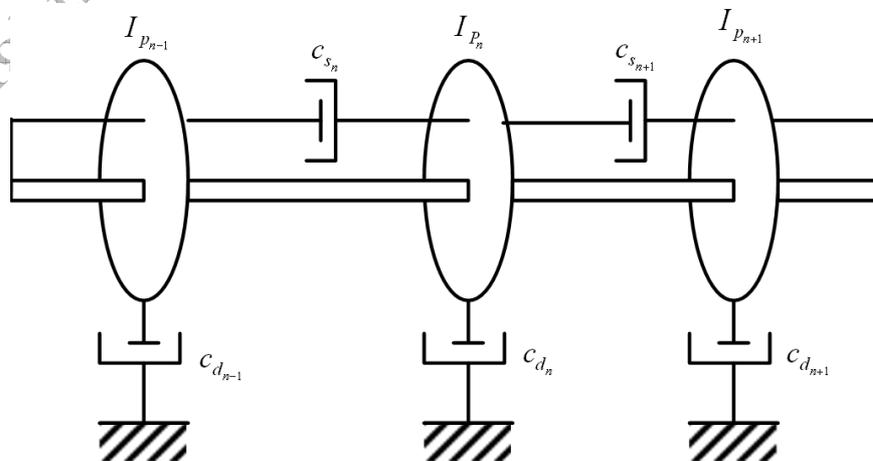
Figure 6.47 General arrangement of multi-DOF rotor system with damping.
