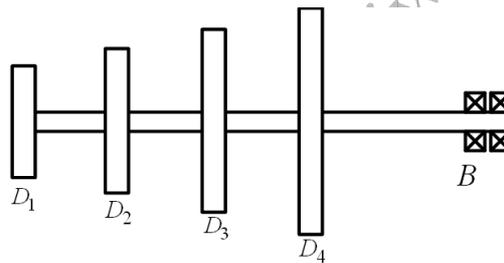
Figure E6.16 A multi-disc overhung rotor
