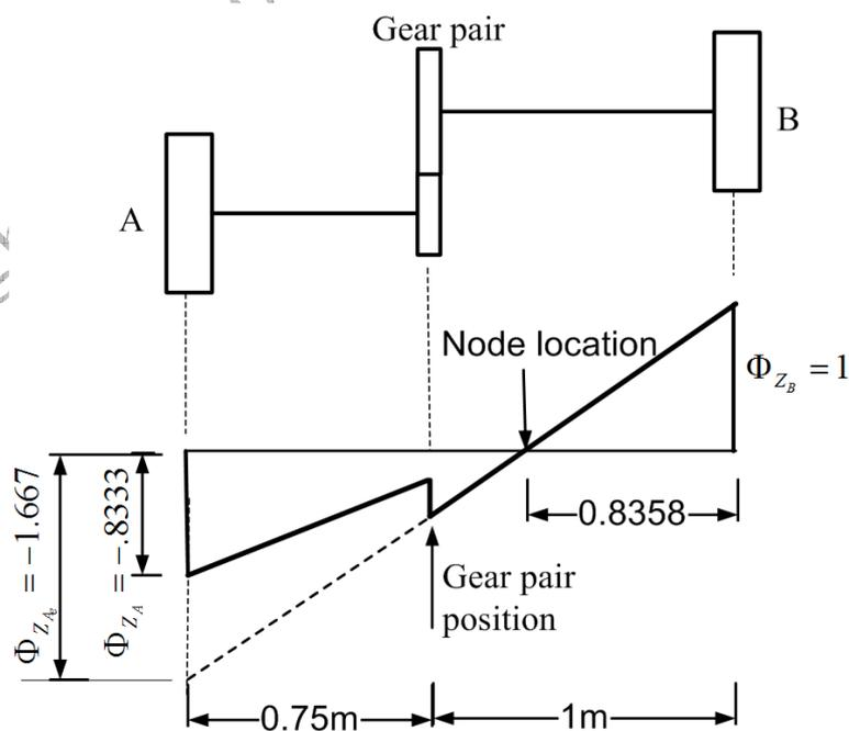
Figure 6.36 The mode shape and the node location in the actual geared system
