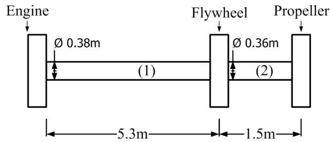
Figure 6.53 A three-disc model of the engine, flywheel and propeller
