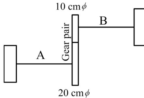
Figure E6.10 A geared rotor system
