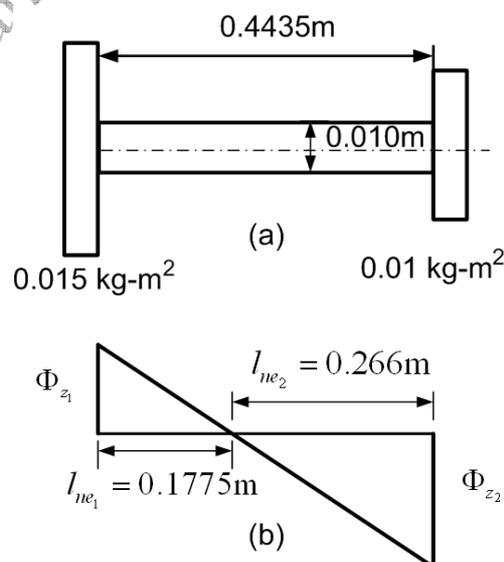
Fig. 6.11 (a) Equivalent system and (b) its mode shape and node position
