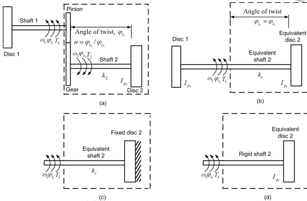
Fig. 6.30 (a) Actual geared system (b) An equivalent system without geared system (c) The equivalent system with disc 2 as fixed and (d) The equivalent system with shaft 2 as rigid
