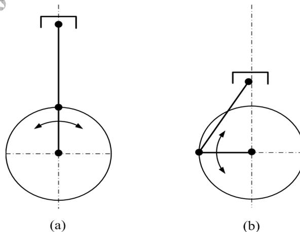
Figure 6.51 An equivalent mass moment of inertia of the piston and the connecting rod
