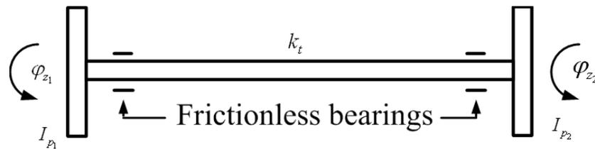
Figure 6.4 A two-disc torsional system
