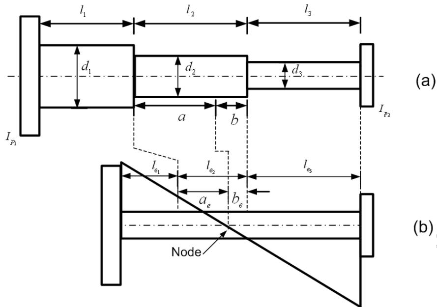
Figure 6.9 Two discs with (a) a stepped shaft (b) an equivalent uniform shaft
