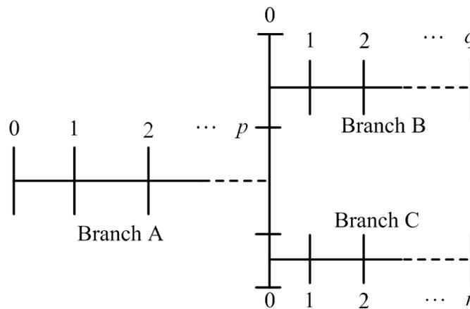
Fig. 6.40 A branched multi-DOF rotor system
