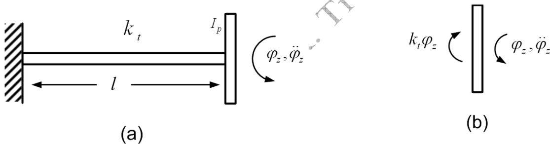
Figure 6.1(a) A single-mass cantilever rotor system (b) A free body diagram of the disc
