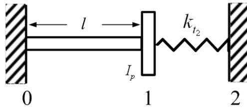
Figure 6.24 A cantilever rotor with a spring at the free end
