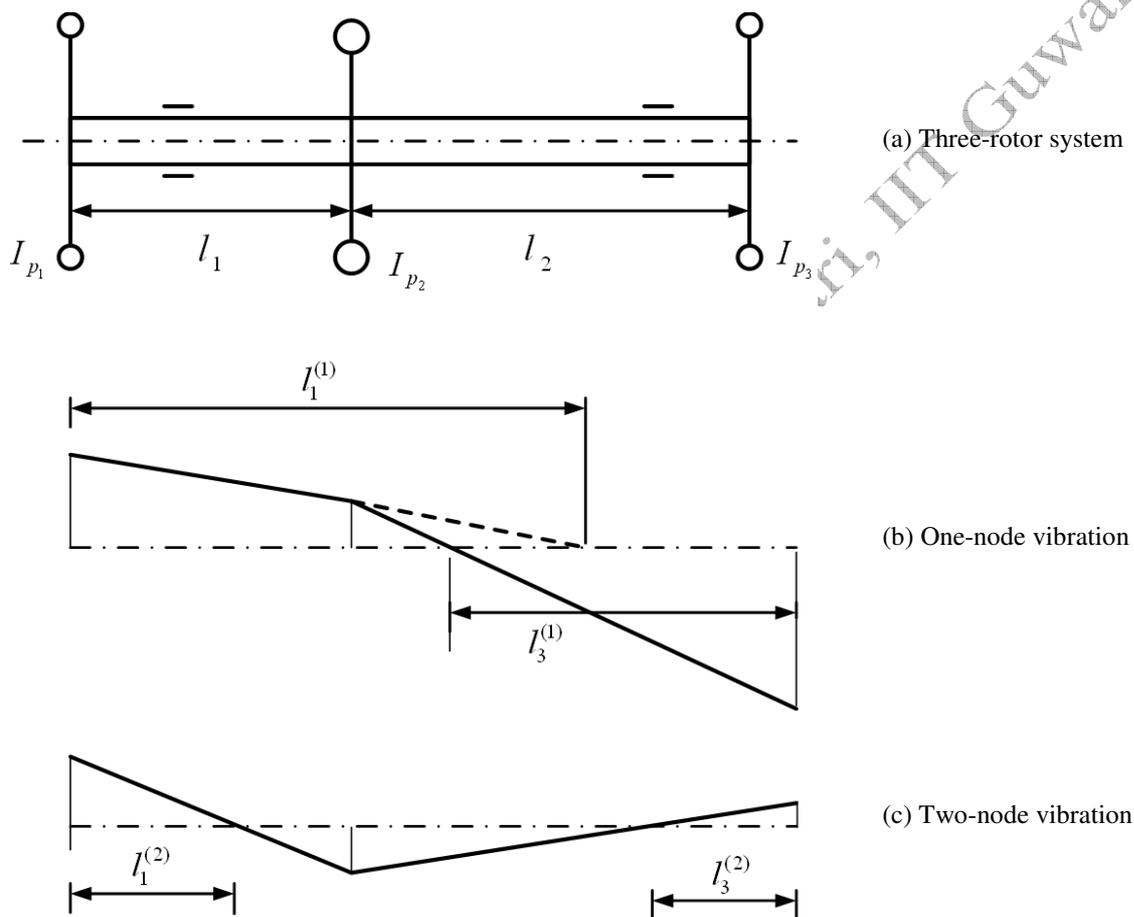
Fig. 6.16 A three-disc rotor system with two possible flexible modes
