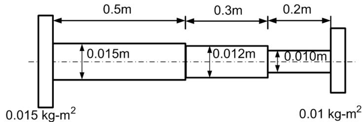
Fig. 6.10 A stepped shaft with two discs
