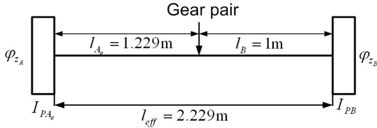
Figure 6.34 An equivalent single-shaft geared system
