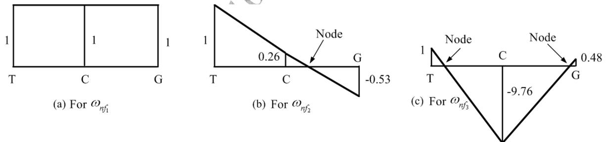
Fig. 6.15 Three mode shapes corresponding to three torsional natural frequencies
