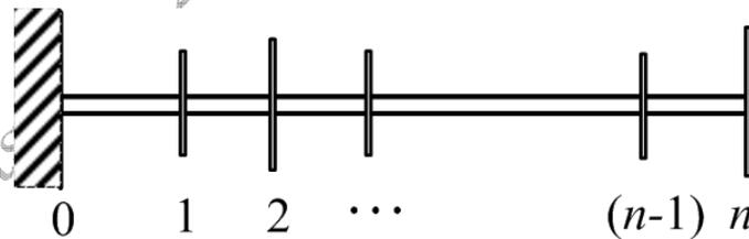
Fig. 6.21 A multi-DOF rotor system with fixed-free boundary conditions
