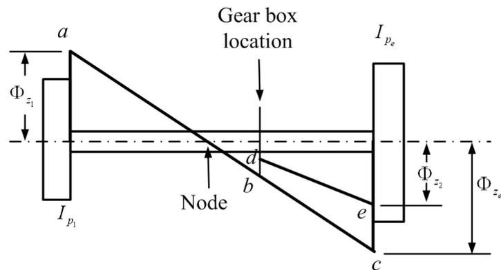
Figure 6.31 The elastic line in the equivalent and original systems
