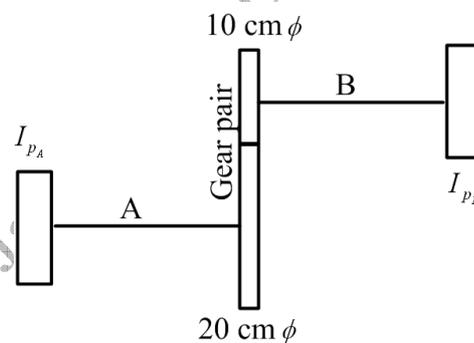
Figure 6.32 A two-disc geared system
