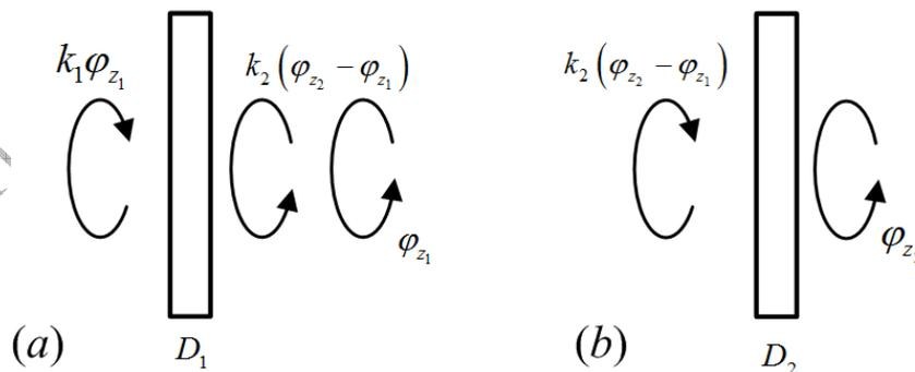
Figure 6.27 Free body diagrams of discs
