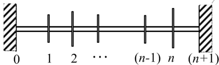
Fig. 6.22 A rotor system with fixed-fixed boundary conditions
