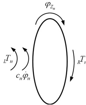
Figure 6.48 A free body diagram of  $r^{\text{th}}$  rotor.
