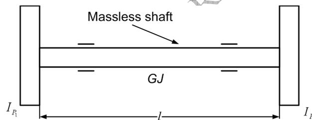
Figure 6.8 A two-disc rotor system
