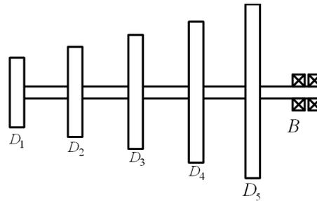
Figure E6.17 A multi-disc overhung rotor
