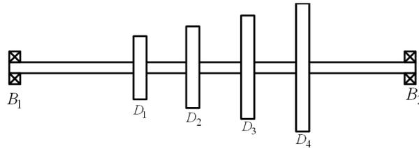
Figure 6.30 A multi-disc rotor system
