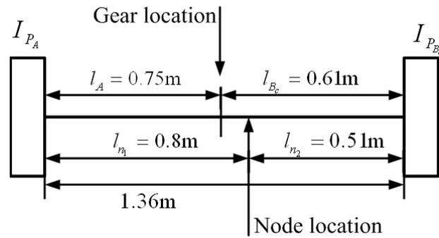
Figure 6.39 Equivalent two mass rotor geared system
