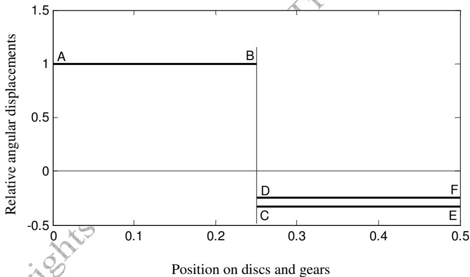
Figure 6.43 Mode shape of the branched system for  $\omega_{nfi} = 0$
