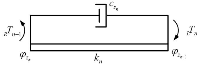
Figure 6.49 A free body diagram of  $n^{\text{th}}$  shaft segment
