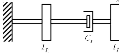
Figure 6.46 A schematic of a torsional vibration damper
