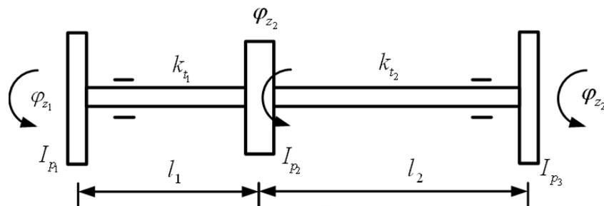
Figure 6.12 A three-disc torsional system
