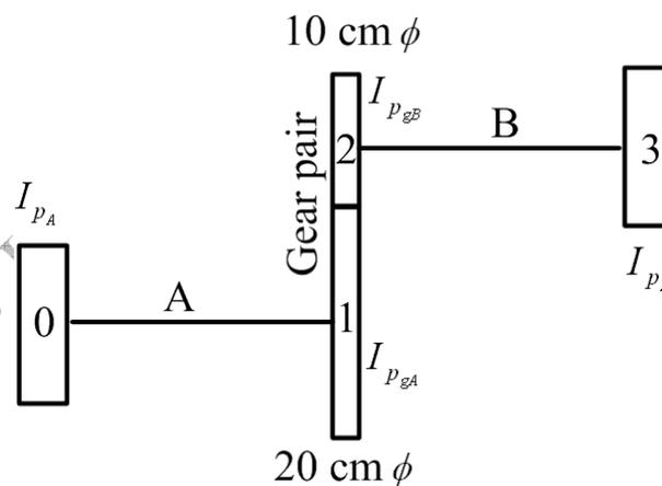
Figure 6.41 Two-discs with a geared system
