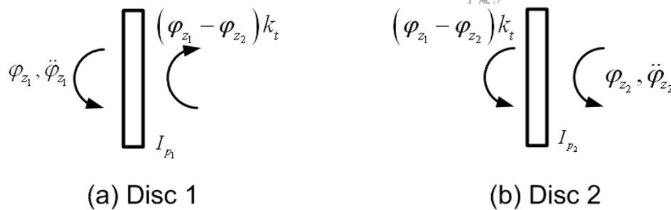
Figure 6.5 Free body diagrams of discs
