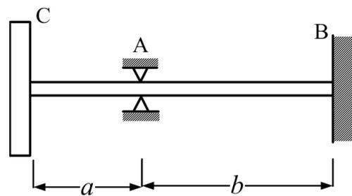
Figure E6.6 An overhung rotor system with an intermediate support
