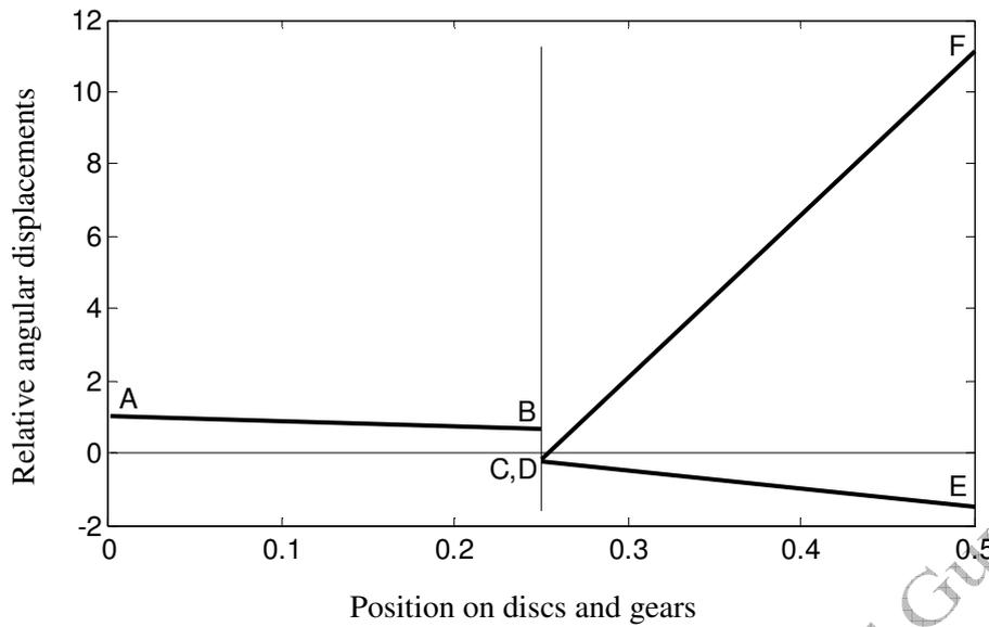
Figure 6.44 Mode shape of the branched system for  $\omega_{nf_2} = 924.4 \text{ rad/s}$
