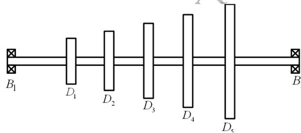
Figure E6.18 A multi-disc rotor system with simply supported end conditions
