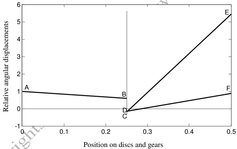
Figure 6.45 Mode shape of the branched system for  $\omega_{nf_3} = 1020.6 \text{ rad/s}$
