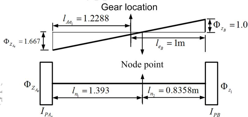
Figure 6.35 Mode shape and nodal point location in the equivalent system
