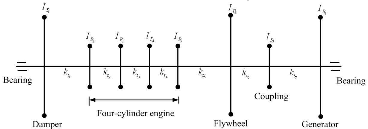
Figure 6.50 A rotor model with  $N$ -disc of a typical reciprocating engine installation
