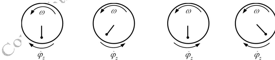
Figure 6.2 Torsional vibrations of a spinning rotor
