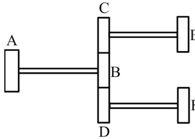
Figure 6.42 A branched rotor system
