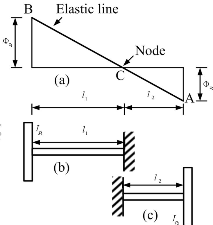
Figure 6.7 (a) The second mode (b) equivalent system 1 (c) equivalent system 2
